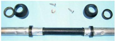
15 Meter Trap after the copper coil was removed. Center insulator was cleaned with alcohol. Aluminum was polished with 600 grit wet/dry sandpaper & water, then cleaned with alcohol. Page 3:
