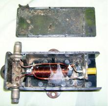
*Picture below:* The same Balun has been cleaned, resoldered, and a new SO-239 connector has been installed. The wires have been painted for illustration to identify the 3 windings.
