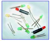
LED's (light emitting diodes) were becoming available in the 1970's at decreasing prices. The light output was very low, in the order of 1 to 7 mcd (milli-candela). Maximum allowed current of 20 mA (milliamperes) was needed for reasonable light output. For battery/portable operation this was significant power drain but better than the available 40 mA incandescent lamp for some applications. A common pilot lamp for decades, #47 pilot
